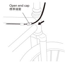
6. Pass the brake inner cable through brake noodle and seat outer casing.
