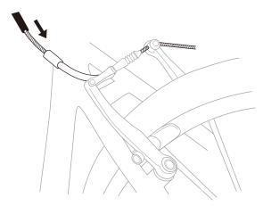
8. Cut off excess inner cable and crimp the cable tip 將多餘的剎車內線剪斷後,套上剎車內線專用線尾帽,並夾緊防止脫落。
